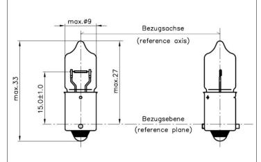
Light center length: 15mm ± 1mm Bulb diameter: max. 9mm
